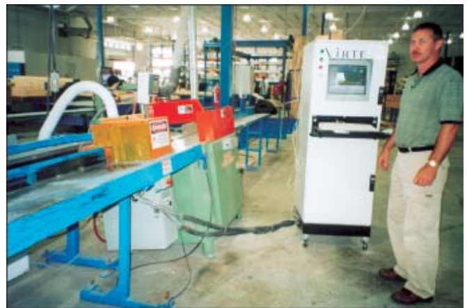
Virtek Visions' Laser MC automated system measures, marks and cuts wall panel parts in a single operation. Laser beams mark each part and maximize yield through optimization.
