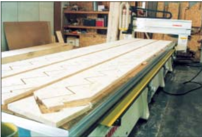
CNC router machine by Thermwall can automatically route stringers for three staircases in a matter of seconds. Super strong stringers are made with LSL engineered lumber.
